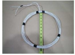
This was made by wrapping the wires around the outside bottom of a 5gal chemical bucket. Tapping the wires as the ring is pulled down off the bottom of the bucket will help keep the wires together. Notice that the lead wires are twisted. This is normally all that you need to test with.
